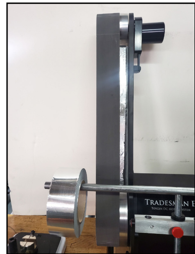
Use of foil tape to reduce static
